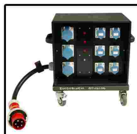
Distribution Box A Input: C-form 63amp / 3 phase Output: 3 x C-form 32amp / single phase 6 x C-form 16amp / single phase 6 x 15 amp outlets
